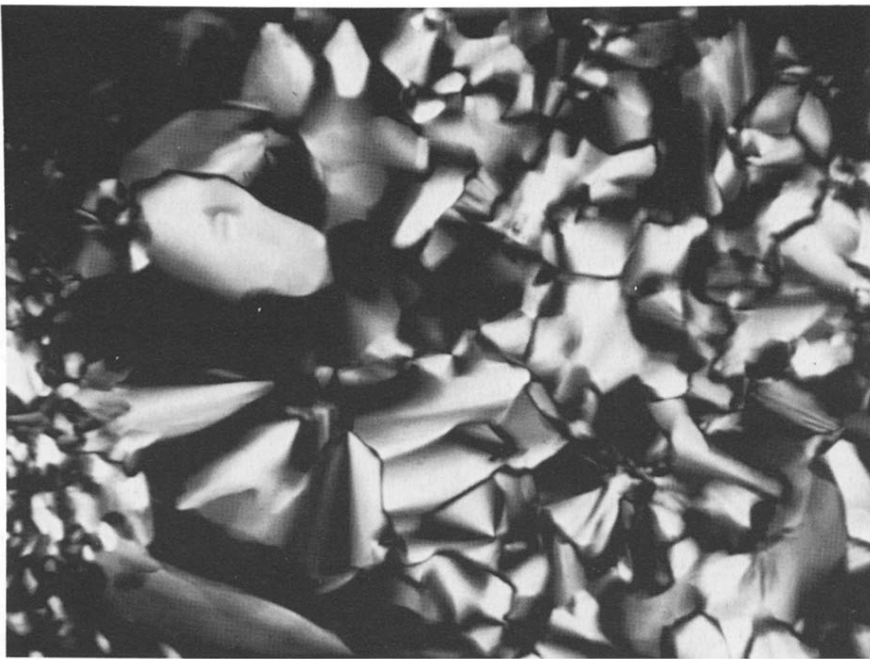
Fig. 3. Texture of smectic phase at 368.4 K for 0.1 mole fraction mixture.
